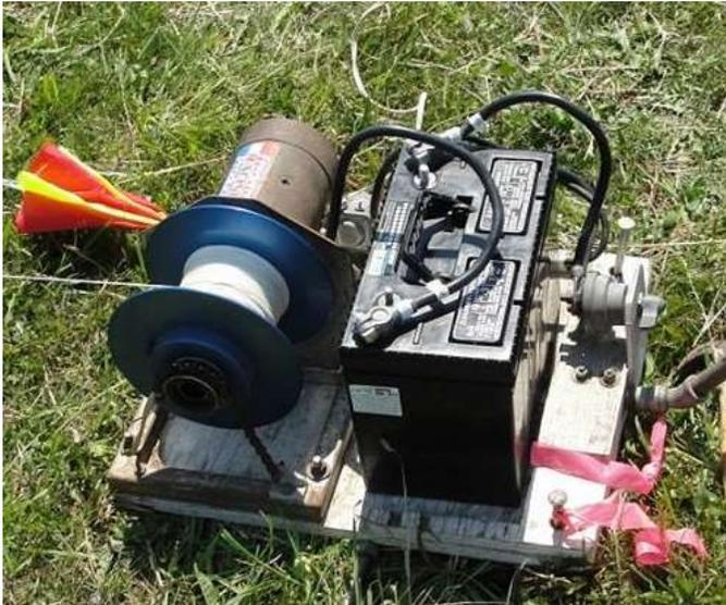
The winch and battery used to launch gliders.
